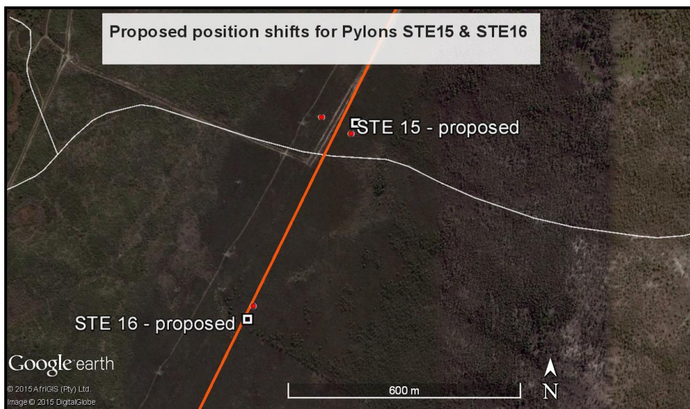
Figure 6: Map showing proposed position shifts of pylons STE15 and STE16. The entire area along this section of the servitude is a High sensitivity area, and the shifts are merely to try and minimise impacts on various threatened plant species.
